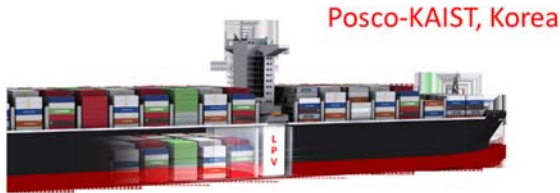
Prismatic tanks take less space than large diameter LNG bullet tanks
