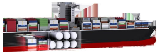
Prismatic tanks take less space than large diameter LNG bullet tanks
